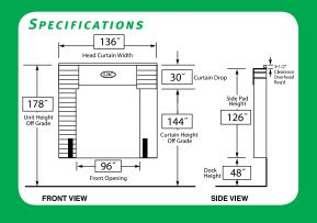
Generally designed to suit 10' wide x 10' high openings. This unit is ideal when full access to the rear of the truck is required. With a standard velcro split head curtain, this unit services a variety of truck heights.
