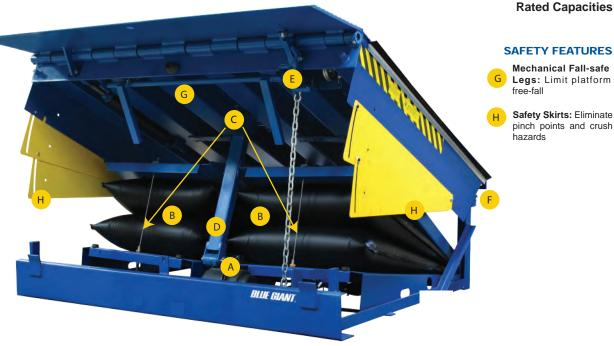
The Blue Giant **U-Series airbag dock leveler** (patent pending) combines our advanced, environmentally friendly air lifting system with the durable structural design that's made us a global leader in the design, manufacture, and distribution of loading dock systems.
