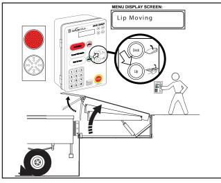
3. Once the lip has deployed, release the 'Lip' button. Both dock leveler and extended lip will descend onto the vehicle load bed. The LCD message will change to 'Deck Moving'. The outside traffic light (optional) remains RED and the control station light (optional) turns GREEN, advising dock staff that loading / unloading operations may begin. NOTE: Ensure that the full width of the lip overlaps the vehicle load bed by a minimum of 4" (102mm).
