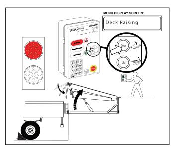
2. When the lip has fully retracted, release the 'Deck' button. The LCD screen will read 'Deck Moving' and the dock will fall back to the stored position with the lip resting in the lip keepers. The LCD message will change to 'Dock Leveler Restored'. The control station light (optional) will change from GREEN to RED,and the outside traffic light (optional) turns GREEN.
